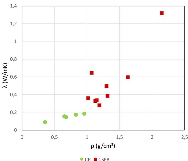
Figure 4. Thermal conductivity as a function of the density. The red square symbols correspond to CSPB specimens and the green circular symbols correspond to CP specimens.
