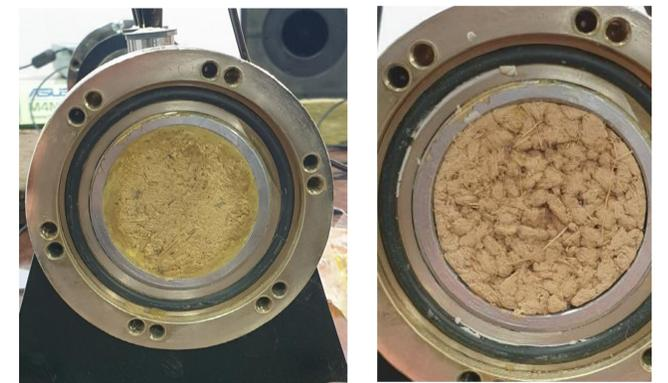
Figure 2. Specimens placed in the impedance tube
