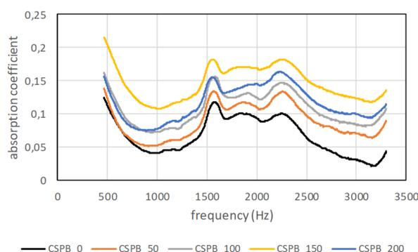
Figure 5. Sound absorption coefficient for the CSPB samples. The curves are an average of 3 specimens.
