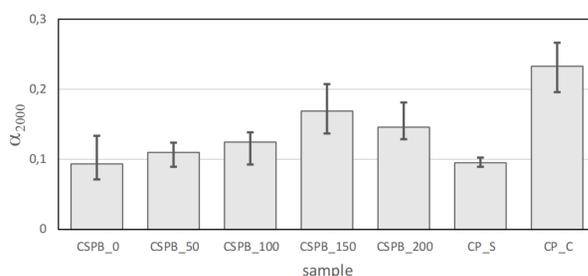
Figure 7. Sound absorption coefficient for frequency 2000 Hz corresponding to all the specimens analysed. The errors are also indicated.
