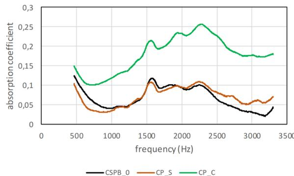
Figure 6. Sound absorption coefficient for the CP samples. The curves are an average of 3 specimens. CSPB\_0 case is included for comparison.
